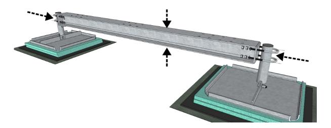
Install 1x back support GR120-16-P53 on each end of the main horizontal beam using M12x40 bolts
