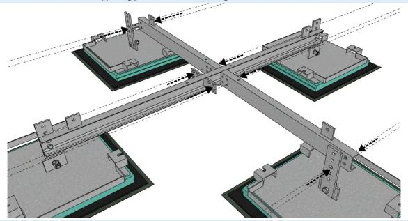
Use 8x M12x50 bolts to connect side hor.beams to the flanges on the main beam
