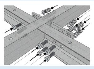
Use M16x50mm bolts to connect other end of the side hor.beam to the supporting panels
